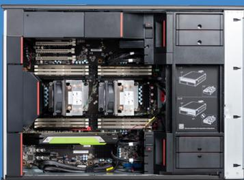
The ThinkStation P900 and P700 Series are built to support dual Intel Xeon scalable processors and up to the new NVIDIA Quadro RTX 8000 graphics inside.
